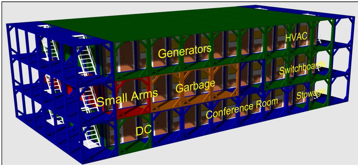
Figure 2: Example of one 40-foot modular support section
