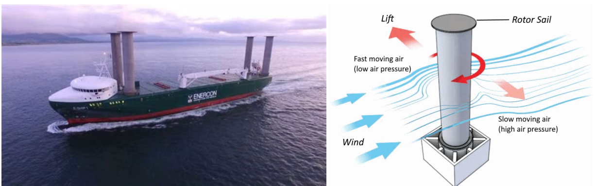
Figure 1: Flettner Rotor Installed on a Vessel (Left) and Description of Magnus Effect (Right)
