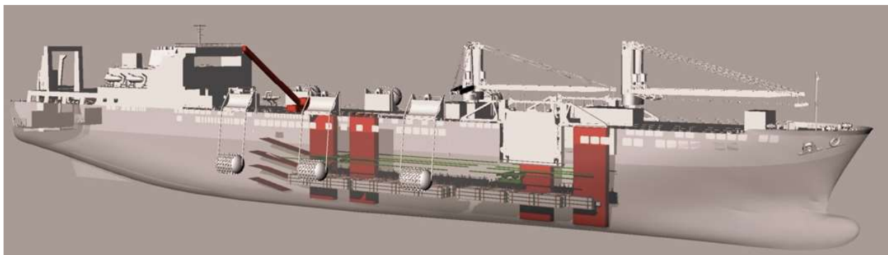
Figure 5: T-AKR Elevator and Hold Concept
