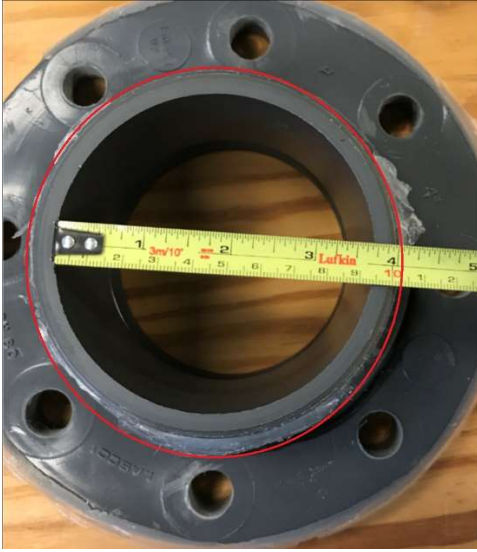
Figure 3-4 The red circle on the left image displays the material that was removed to allow subjects with average measurements to participate in the experiment. Image on the right portrays the flange mounted onto the test tank.
