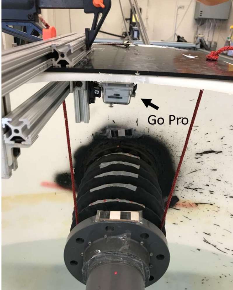
Figure 3-5 GoPro mounted 33 cm above and positioned in the middle of joint
