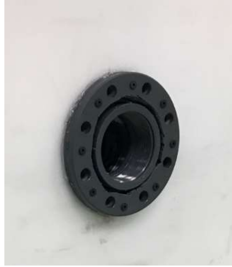
Figure 3-4 The red circle on the left image displays the material that was removed to allow subjects with average measurements to participate in the experiment. Image on the right portrays the flange mounted onto the test tank.
