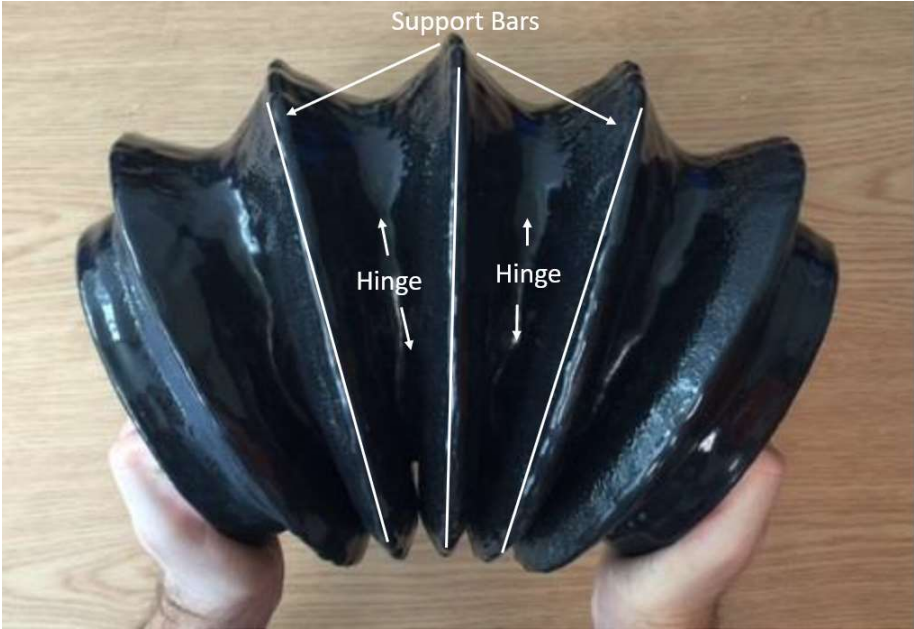
Figure 2-4 Prototype elbow joint provided by Midé including PVC hardware required for mounting and to sealing
