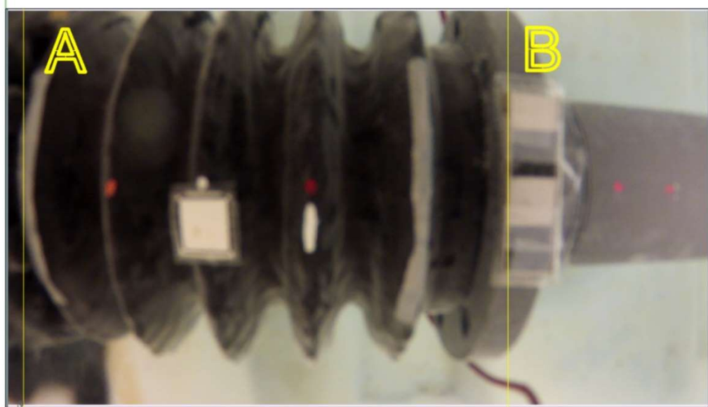
Figure 4-3 “A” is fixed reference plane while “B” is unconstrained and will be used to measure angle the joint traveled through
