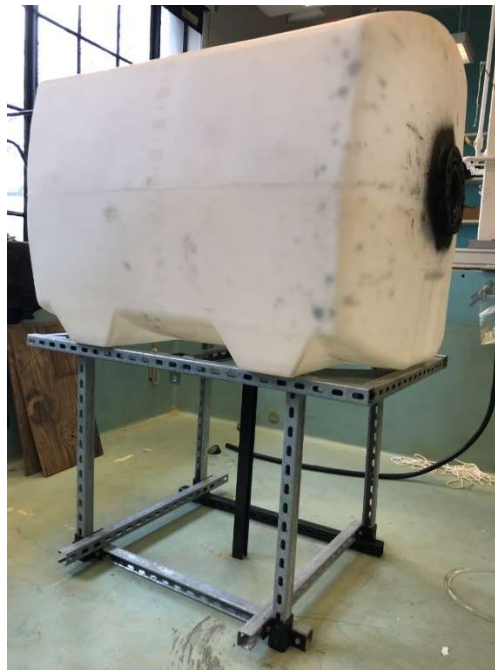
Figure 3-2 Stand constructed so that columns are placed below footpads which reduces beam loading and allows a safety factor of 6 to be achieved for column buckling
