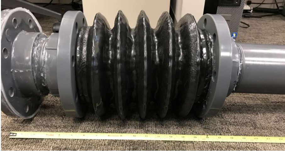
Figure 2-4 Prototype elbow joint provided by Midé including PVC hardware required for mounting and to sealing
