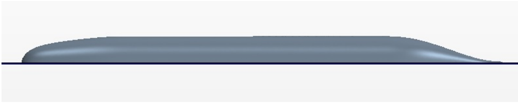
Figure 3-3: The CFD simulation domain utilizes symmetry to only model half of the vehicle in order to reduce the computational expense of the simulation.
