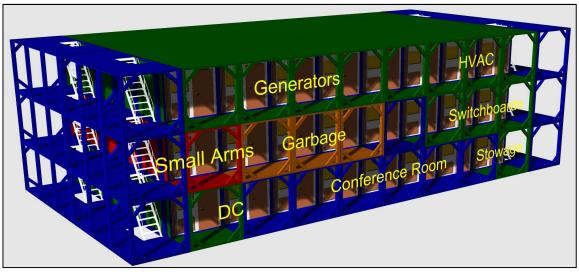
Figure 2: Example of one 40-foot modular support section
