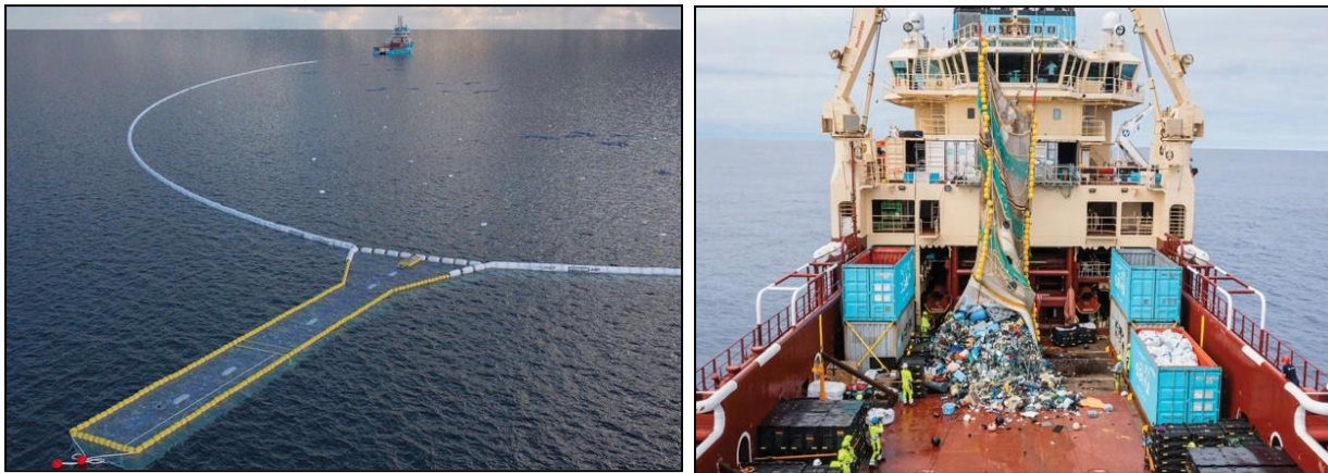
Figure 1: The Ocean Cleanup's Jenny 002 System (Left) and Retention Zone on Aft Deck (Right)
