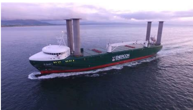
Figure 1: Flettner Rotor Installed on a Vessel (Left) and Description of Magnus Effect (Right)
